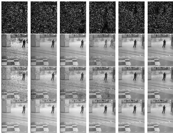
Figure 3. Results for background modeling with virtual pan. The first row shows the known entries used for training in frames 40, 70, 100, 130, 170, 200. The remaining rows show the results obtained by PRMF, GRASTA and our method, respectively.
