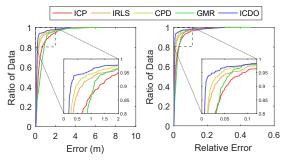
Figure 5. Results of ETH laser registration dataset in cumulative plots. (Left) Absolute registration error. (Right) Relative error.
