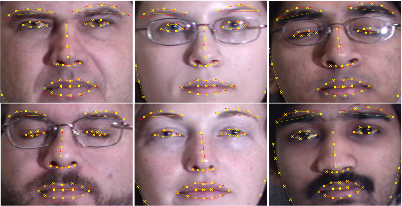
Figure 7. Red dots represent the initial manual labeling. Yellow crosses are the landmarks re-labeled with PKPCA (better seen in color).
